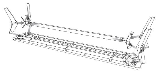
1. Install the legs into the bench top like picture above and tighten with bolt ring and nut. Please make sure the code of bolt.
