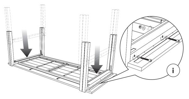
1. Install the frame legs as picture above and tighten with bolts, ring and nut as in detail (i)
