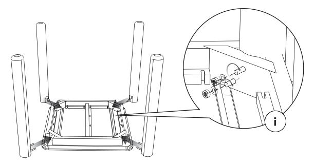
1. Install the legs into the table top as picture above and tighten with nut and rings as in detail (i)  $\frac{1}{2} \left( \frac{1}{2} \right) \left( \frac{1}{2} \right)$
