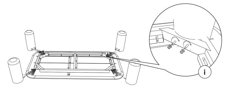
Install the legs into the table top as picture above and tighten with nut and rings as in detail (i)
