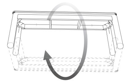
2. Rotate the bench into its right position as in picture above.
