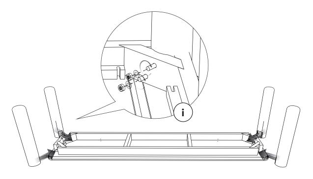
1. Install the legs into the bench top as picture above and tighten with nut and rings as in detail (i)  $\frac{1}{2} \left( \frac{1}{2} \right) \left( \frac{1}{2} \right)$
