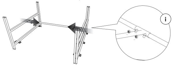
1. Install the frame support into the legs like picture above and tighten with rings and nuts as in detail (i)
