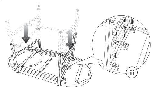
2. Install the legs into the table top like picture above and tighten with bolts and rings as in detail (ii)  $\,$
