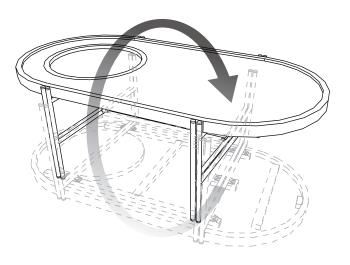
3. Rotate the table into its right positions.
