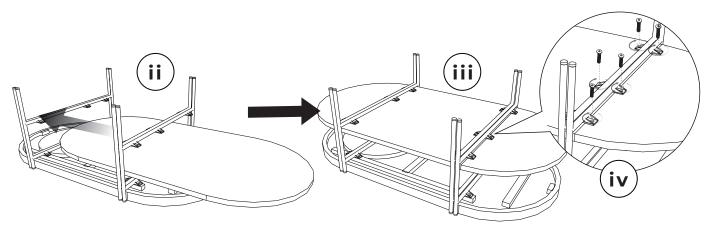
2. Place the second table top like picture above (ii) into its right position and tighten the top into the frame legs like picture above (iii) and tighten with bolts and rings as in detail (iv)
