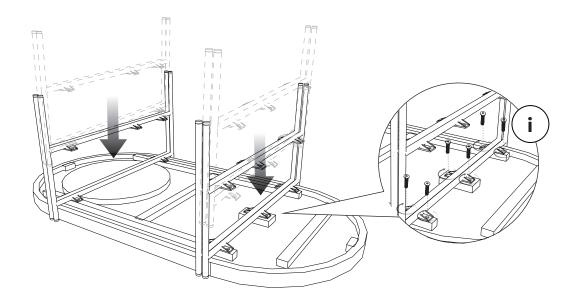
1. Install the legs into the table top like picture above and tighten with bolts and rings as in detail (i)
