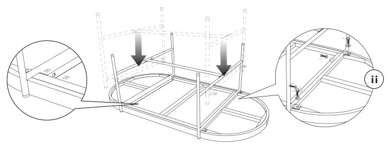
2. Install the legs into the table top like picture above and tighten with bolts and rings as in detail (ii). See the code is correctly paired.
