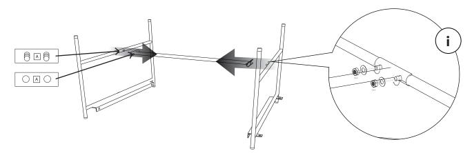
1. Install the frame support into the legs like picture above and tighten with rings and nuts as in detail (i)  $% \left( {\left( {{{\left( {1 \right)} \right)}} \right)} \right)$
