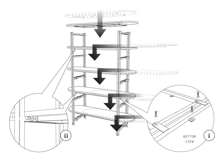
1. Place the shelves as in picture above and tighten with bolts and rings as in detail (i) and (ii)
