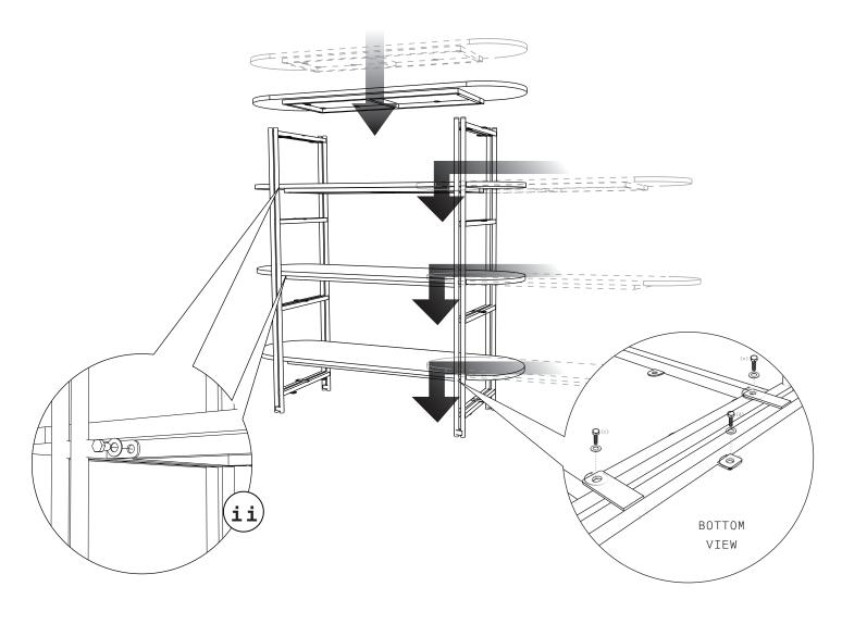
1. Place the shelves as in picture above and tighten with bolts and rings as in detail (i) and (ii).
