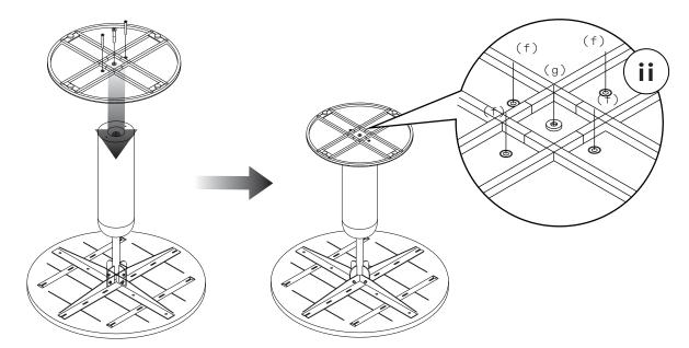
3. Install the iron bullet leg into the wooden bullet and tighten with screw as in detail (ii)
