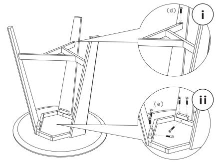
2. After all legs are in right position, tighten the leg into table top and leg connector with hex screws as in detail (i) and (ii)
