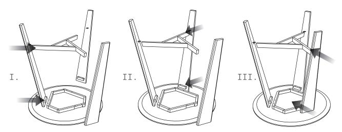
1. Put the leg into table top together with leg connector as in picture above (I, II, III) into its right position but keep them loosy.
