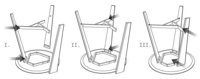
1. Put the leg into table top together with leg connector as in picture above (I, II, III) into its right position but keep them loosy.
