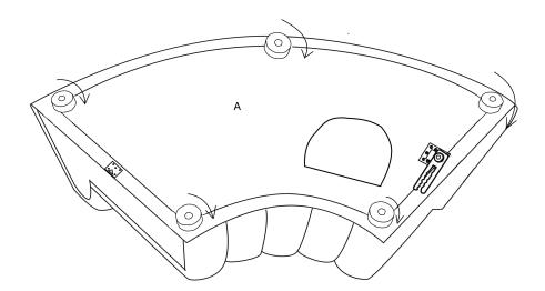
Attach the legs to the bolts, tighten the legs by rotating them clockwise.
