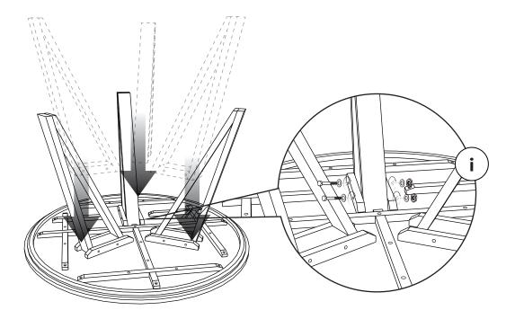
Install the legs into the table top like picture above and tighten with bolts, rings and nuts as in detail (i)
