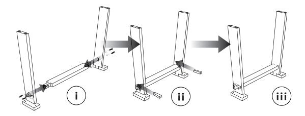
Stack the legs with leg connector and tighten with hex screw (i) and lock with wooden locker (ii) as in detail above until its installed (iii)
