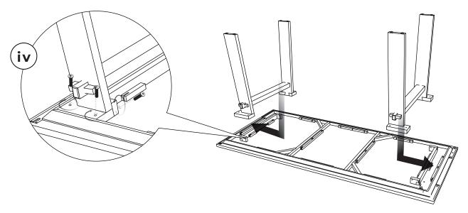
2. Instal the legs into the table top and tighten with hex screw as in detail (iv)  $\,$
