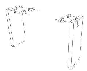
Install Wooden connector on the legs into its right positions like picture on the left and tighten with bolt and rings.
