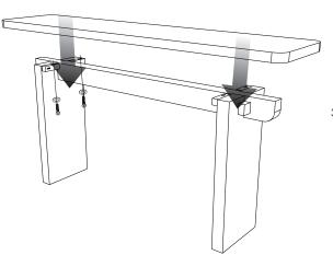
3. Install the table top into the legs like picture on the left and tighten the top table from below with bolt and rings through the wooden connector.
