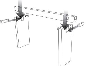
2. Install the beam into the legs and lock it with wooden locker as picture on the right.
