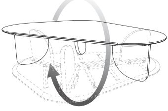
3. Rotate the table into its right position.
