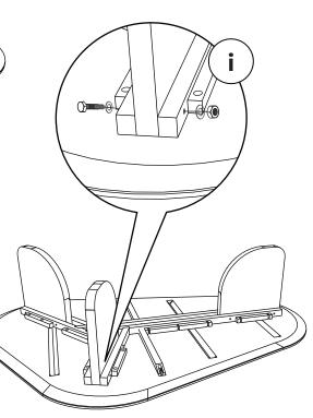
Tighten the legs with bolt ring and nut as in detail (i)
