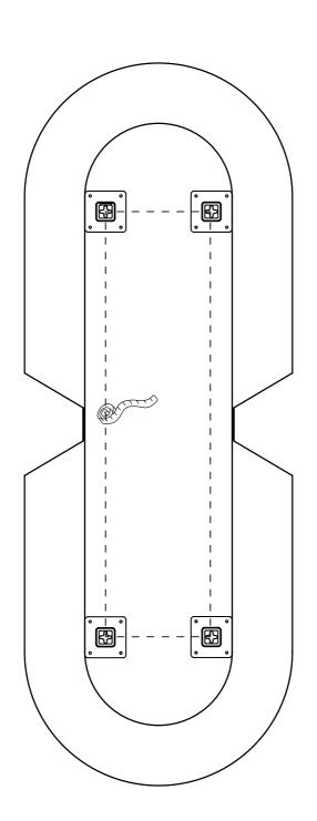
Use minimum 2 brackets for wall mounting. 3rd and 4th bracket is optional.
