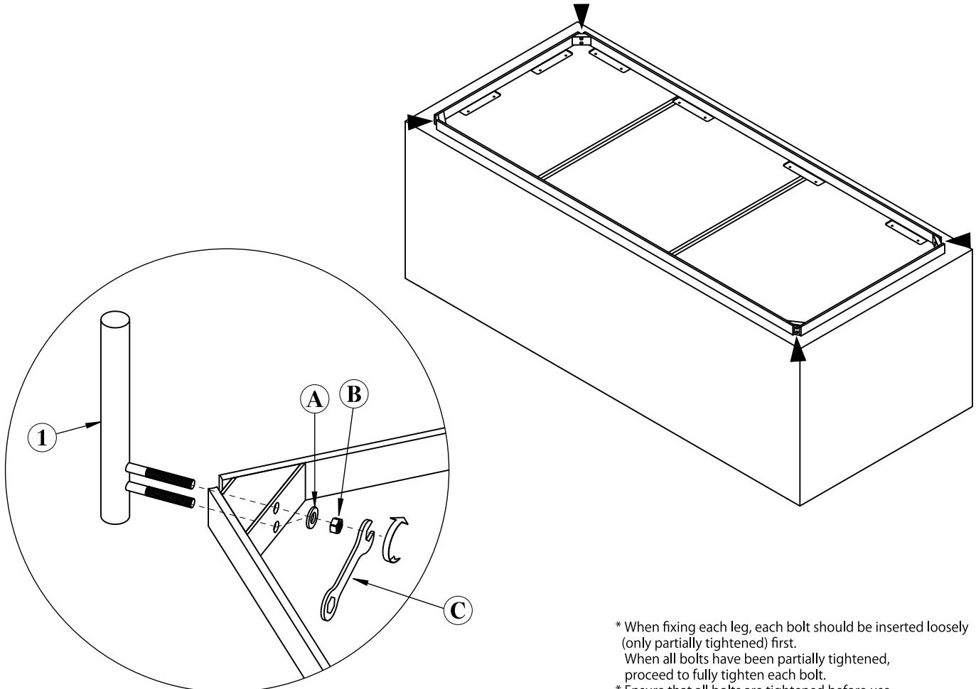
\* When fixing each leg, each bolt should be inserted loosely (only partially tightened) first.
