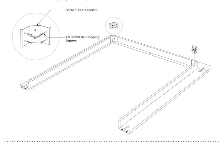
Position both Tail Base (Left & Right) as shown and secured with 4 sets of M8 x 20mm Hex Head Screw with  $\emptyset$  13/ $\emptyset$ 8 x 2mm Washer.
