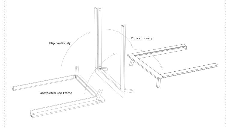
Position completed Bed Frame to Headboard as shown.
