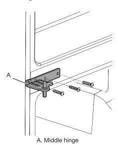
Lift freezer door from the bottom hinge pin.
