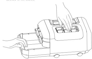
Manual ice maker assembly can be taken out of the freezer when ice is not required to make more compartment in freezer.
