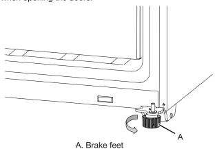
**IMPORTANT:** If you need to make further adjustments involving brake feet, you must turn both brake feet same amount to keep the refrigerator level.
