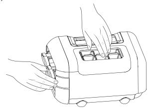
Lift ice container slightly and pullout ice container to get access to ice cubes.
