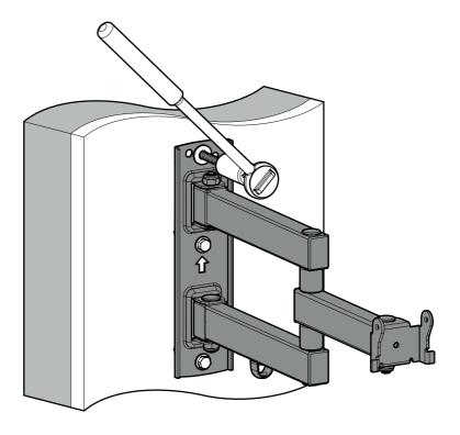
i Check the wall plate is perfectly level. Adjust or re-fit if required.
