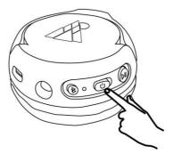
When activating, the LED light next to the on/off button, as well as the light on the side of the speakers, will turn on. If you are wearing the headphones, you will hear an ascending tone.
