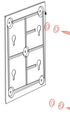
Use screwdriver to secure the mounting plate on the wall with screws.
