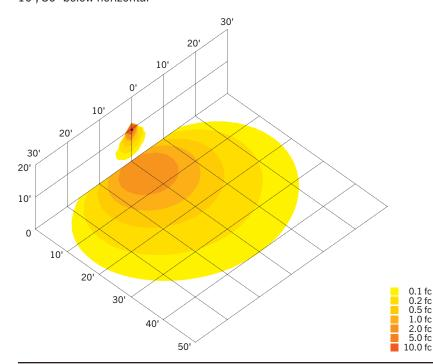
Ground mounted at 6" above ground, 10º above horizontal, shining towards building exterior
