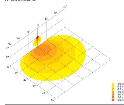
Ground mounted at 6" above ground, 10° above horizontal, shining towards building exterior wall at 8' away
