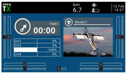
Top menu bar: The default top menu bar displays speaker volume, remote control battery level, receiver signal strength (RSSI), and time and date. Batt is a custom top display remote control voltage; users can also add other display information.
