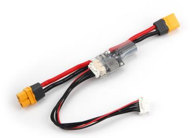
PM02D provides regulated power supply for your Pixhawk® 5X from the battery, as well as current consumption and battery voltage measurements, all through a 6pin cable. The on-board switching regulator outputs 5.2V and a maximum of 3A from LiPo batteries up to 6S. The Power Module comes completely assembled with XT60 connectors, wrapped in shrink tubing for physical damage protection.
