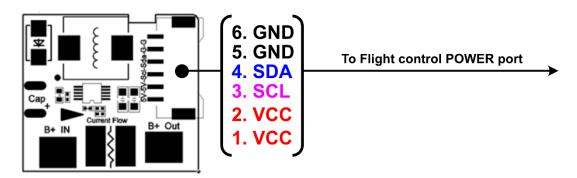
**Note**: PM02D does not require users to set the voltage divider and the current divider ratio. With the default setting parameters, the voltage and current measurement accuracy can be better than 5%.
