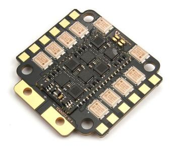
F4 MCU @150Mhz / Metal-Cased MOSFET / PWM output up to 96K / 4~6S / BLHELI32 The all new Tekko32 Metal is the first 4in1 ESC in the market to adapt the fast F4 MCU. Powerful & reliable metal-cased MOSFET 4in1 ESC with smooth control and quick response.
