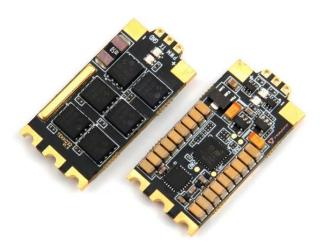
Tekko32 F4 45A ESC is the latest BLHeli32 ESC from HolyBro. The Tekko32 ESC runs in conjunction with an ARM 32bit compatible F4 MCU. It can run input signals with lower latency, at faster rates, smooths out the RPM band, is capable of both voltage and current monitoring and limiting, as well as offering customization of the brake on stop force. The Tekko32 ESC has a lot of room to grow and wide compatibility range with future products.
