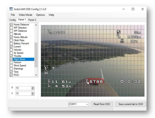
To edit the elements displayed on the screen, select the element you want from the list on the left hand side and then drag it on the screen to the position you prefer, the item will be highlighted in red as shown. For reference the default layout is shown in the image.
