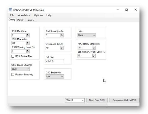
In the first tab called 'Config' you can change the units, warning levels and the channel on the flight controller that will cause the two setup OSD screens to 'toggle'. Disable this if you are not planning on having two different OSD screens. Remember to select the 'Save Current Tab to OSD' in the bottom, right corner to make sure you don't lose any of your changes.
