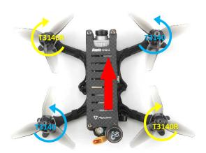
The default motor directions for a Cleanflight or Betaflight quadcopter are shown to the left. Based on this, the correct way to install the props is as shown.
