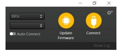
If you don't see DFU in the pulldown menu, then either the board didn't detect that you had the bootloader button pressed or your drivers are not installed correctly. If you don't see DFU in the pulldown menu, you cannot flash new firmware to the board. It won't work.
