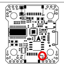
Some ESCs support a feature called ESC Telemetry. This feature allows the ESC to report data such as motor RPM and amps being used by the ESC back to the flight controller. The main advantage of this feature is when the flight controller (such as the Kakute) does not have built-in current monitoring. In this case, the FC can gather current consumption data from the ESCs.
