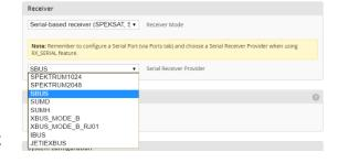
receivers use iBus. These are the most common serial receiver types that are likely to be encountered.
