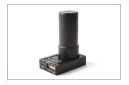
3) <u>H-RTK M8P Base (SKU12021) -</u> The board is the same as number 2 above, but it is equipped with a high-gain antenna. This model is best suited to use as base station. The search speed and positioning accuracy are the highest among the three models.
