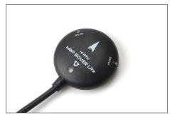
2) <u>H-RTK M8P Helical (SKU12020)</u> - This model uses a helical antenna, which has better performance than the lite version. This model can be used both on rover (aircraft) or as base station. The aluminum alloy shell design also has a integrated safety switch and a tri-colored LED indicator, and it is compatible with the open source *Pixhawk* series flight controller.
