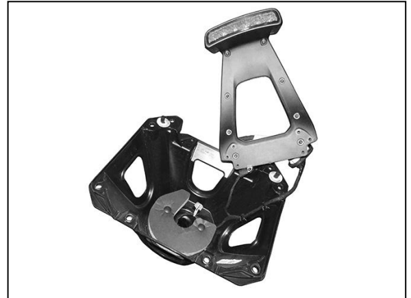
(Fig 21) Models with camera, pull camera assembly out of back of spare tire mount
