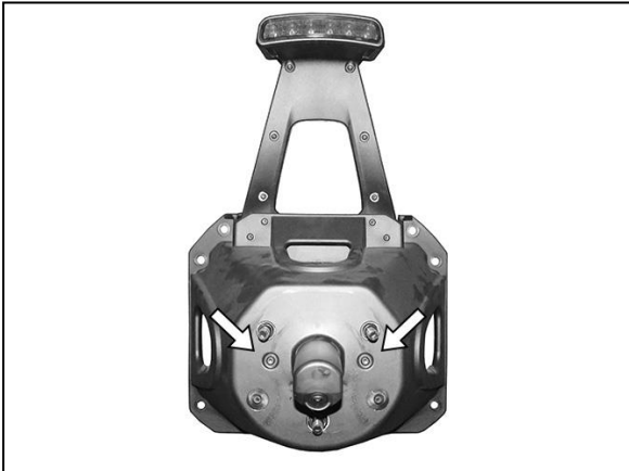
(Fig 20) Models with camera, remove the (2) screws attaching camera housing to spare tire mount (arrows)
