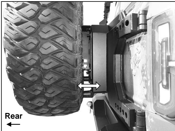
(Fig 32) Adjust rubber bumpers in or out to support the spare tire
