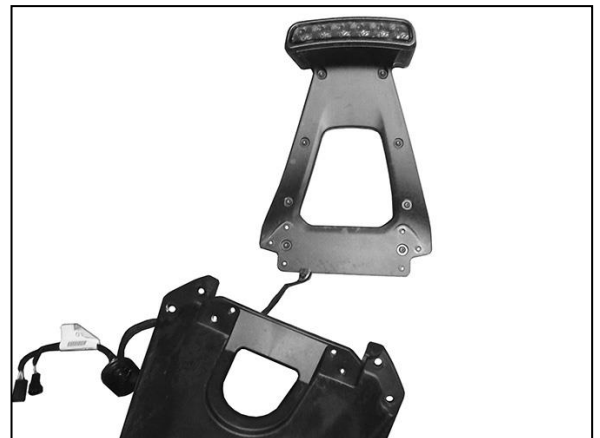
(Fig 18) Remove the brake light assembly from the top of the spare tire mount
