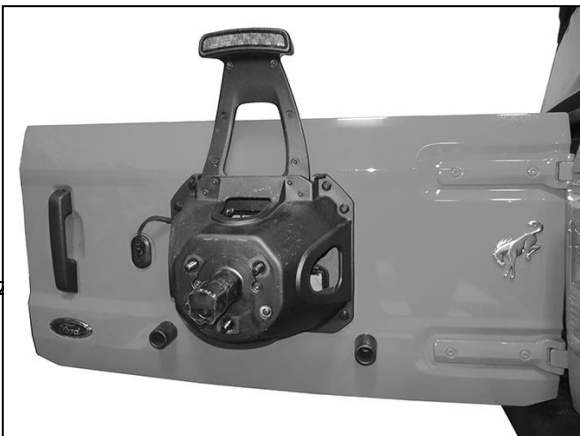
(Fig 3) Remove tire mount from rear door
