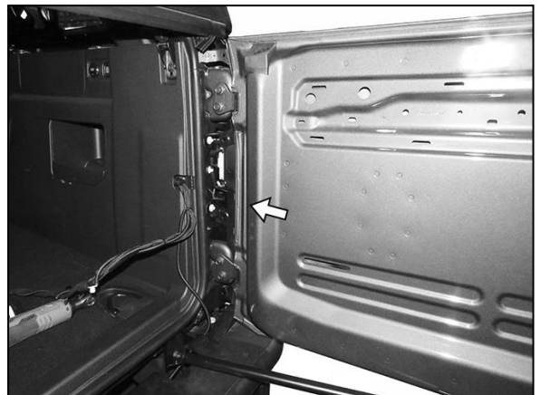
(Fig 4) Remove the plastic cover (arrow). Remove inner wiring harness from rear door
