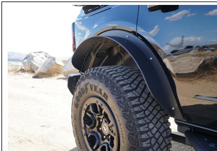
(Fig 7) Level and adjust the Fenders and tighten all hardware. (Passenger/Right side shown)
