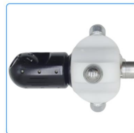
3. screw the 3 white screw on the protective case, until it was fixed on the camera head
