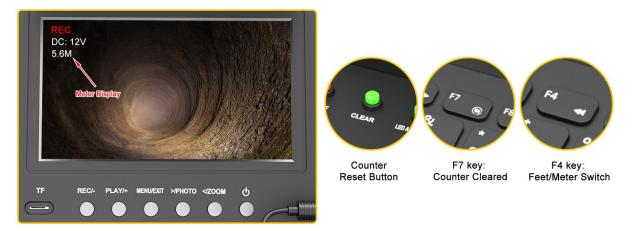
Before using this function, please press the CLEAR button or F7 key to clear the counter information. You can toggle the display in feet or meters by pressing the F4 key. It will start counting feet/meters when the coil rotates, and display it on the screen in real time.
