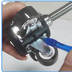
2. put the camera protective case on the camera head
