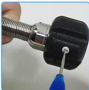
2. put the camera protective case on the camera head
