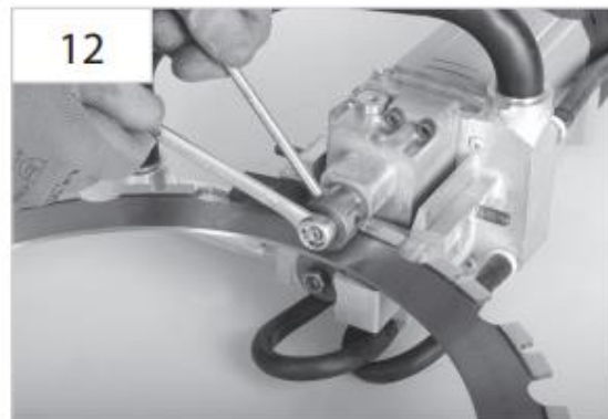
12 Tighten the smooth drive roller. Tool: 1/2" spanner and a punch
