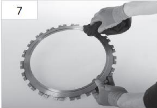
7 Clean both sides of disk grinding ring thoroughly.
