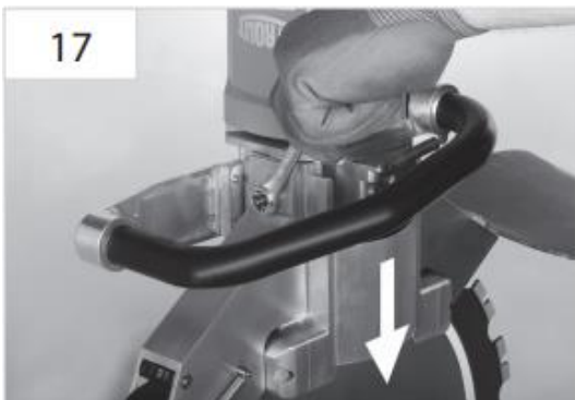
Place housing onto edge of workbench, then push and hold down. Tighten disk guard. Tool: 1/2" spanner
