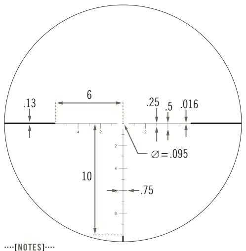
Subtensions are measured in MOA and correspond to magnification at 40x.  $\varnothing$ =Diameter
