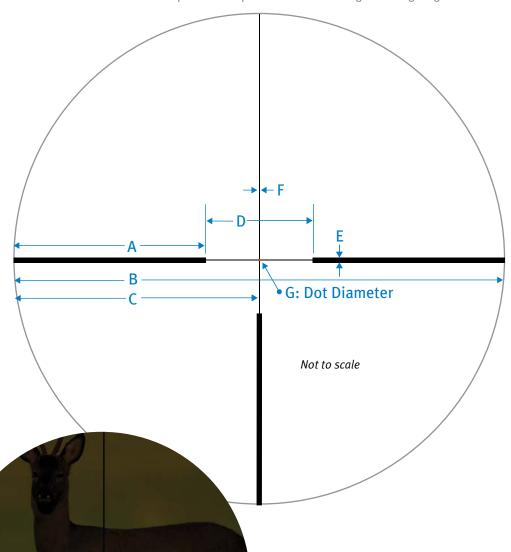
The illuminated center dot provides a precise aiming point at dawn, at dusk, and in other difficult light when black crosshairs can disappear against the dark body of an animal.
