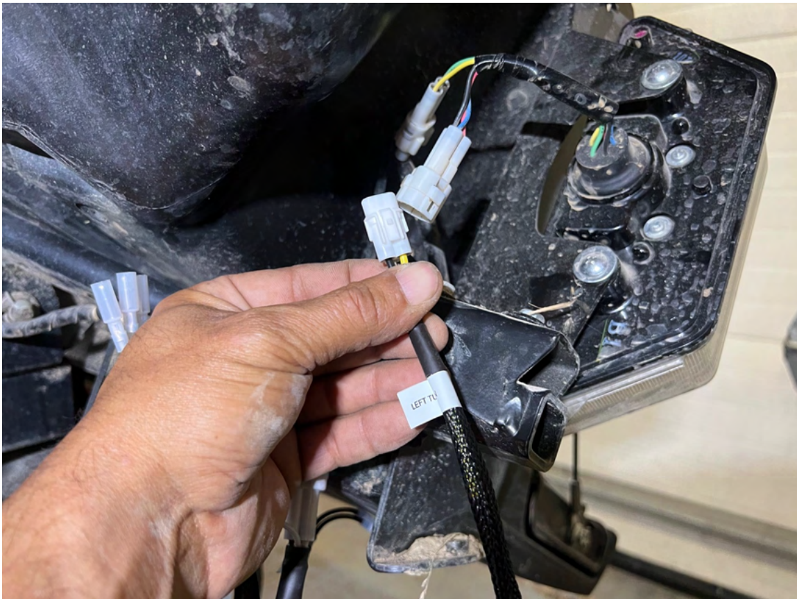
4:2: RUN THE TURNPRO TAILLIGHT HARNESS TO EACH OF THE "LEFT & RIGHT TURN" TAILLIGHTS
