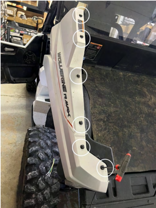
3: REMOVE DRIVERS SIDE BED PANEL Using a #4 Allen remove the 11 bolts.
