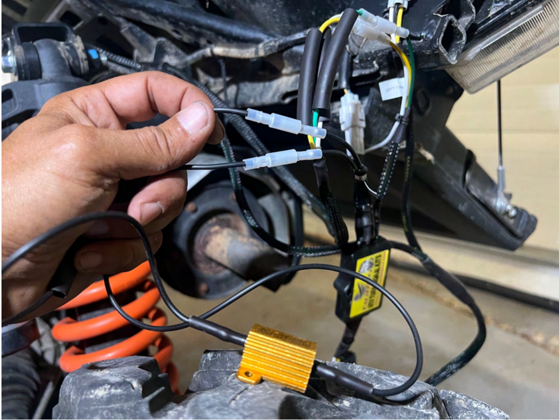
FIGURE 6: SCREW LOAD RESISTOR ONTO THE METAL PART OF FRAME NOTE: DO NOT MOUNT TO PLASTICS FOR RESISTOR WILL GET WARM.
