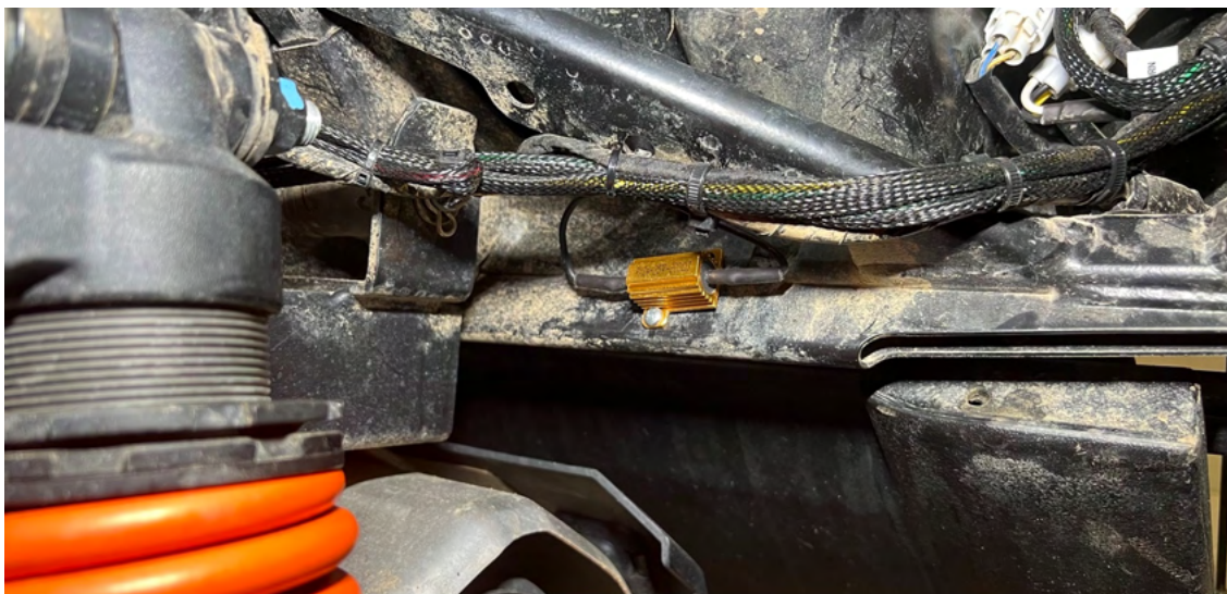
FIGURE 6: SCREW LOAD RESISTOR ONTO THE METAL PART OF FRAME NOTE: DO NOT MOUNT TO PLASTICS FOR RESISTOR WILL GET WARM.
