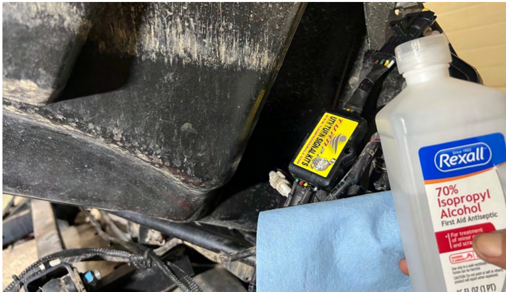
FIGURE 6:1: CLEAN AREA WITH RUBBING ALCOHOL INSIDE OF TAILLIGHT HOUSING AND SECURE PLUG & PLAY MODULE TO THE SIDE WITH THE ADHISIVE TAP.
