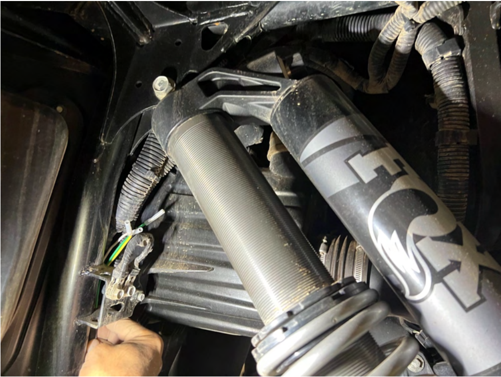
FIGURE 3:7: Finish running rear harness alongside of factory harness to rear of machine (Driver's Side Taillight). "Pictured Below"
