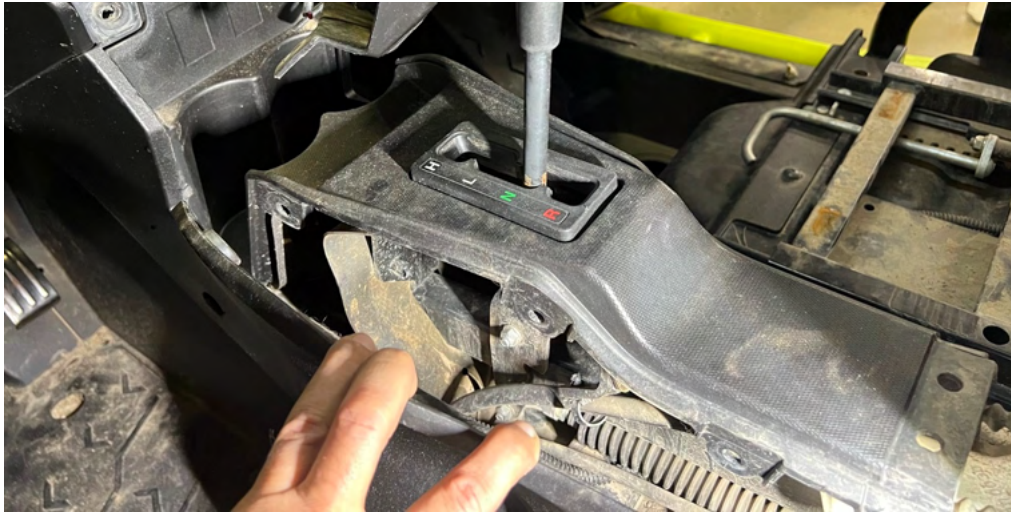
FIGURE 3:2: Locate panel cover on the passenger's side of center console & remove the (3) body clips for access. “Pictured Below”
