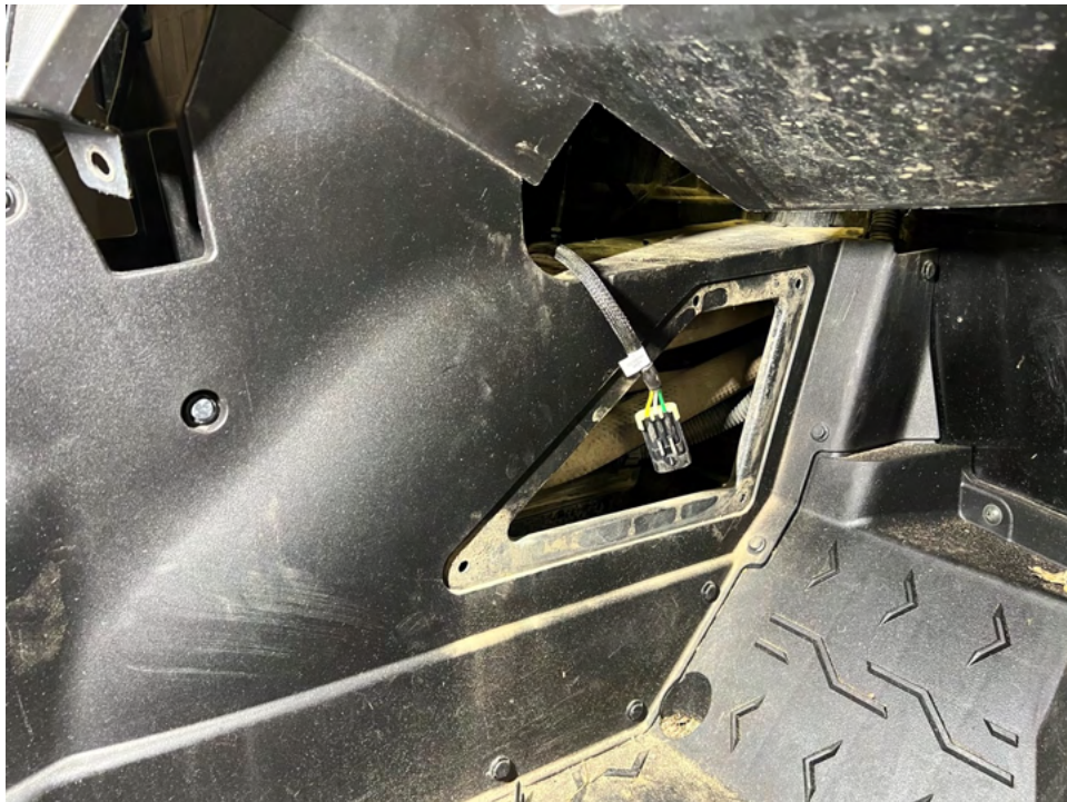
FIGURE 3:4: PHOTO SHOWING REAR HARNESS CONNECTOR PLUG THAT GOES UP TO DASH SWITCH (DASH HARNESS)
