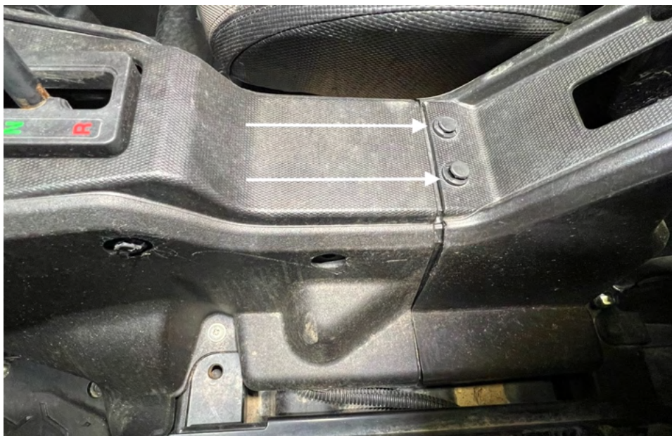
FIGURE 2: REAR CENTER CONSOLE REMOVAL Remove the (2) push pins "Pictured Below."
