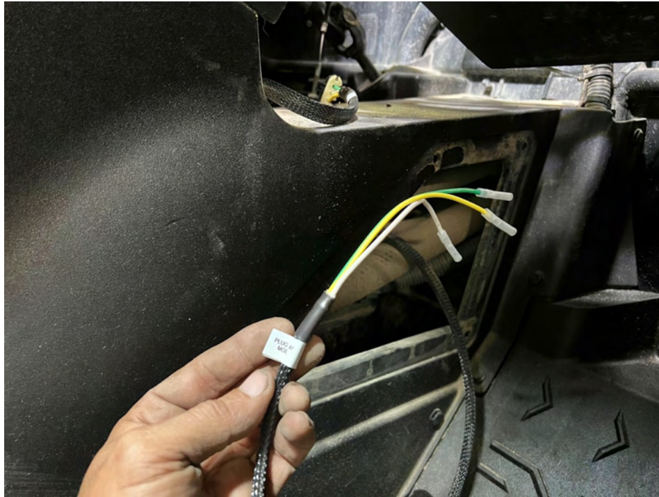
FIGURE 3:4: PHOTO SHOWING REAR HARNESS CONNECTOR PLUG THAT GOES UP TO DASH SWITCH (DASH HARNESS)
