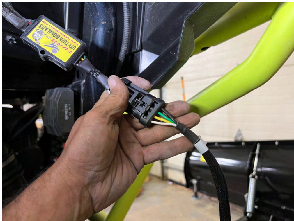
INSTALL 4PIN PLUG TO MATCHING CONNECTOR OF PLUG & PLAY MODULE
