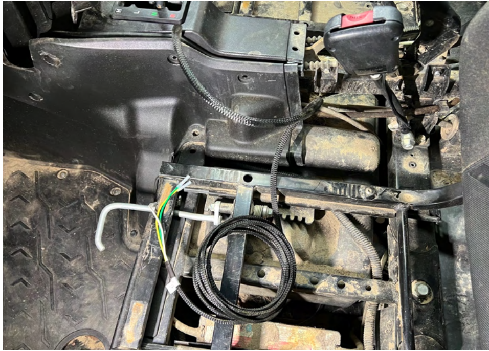
FIGURE 3:6: Run rear harness along side of factory harness out to the rear of machine. (Pictured Below)
