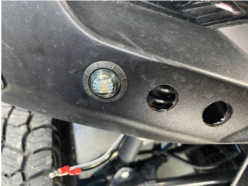
5:4: Wire LED's to harness as followed > BLACK TO BLACK / Harness WHITE TO WHITE as seen in FIGURE 5:3
