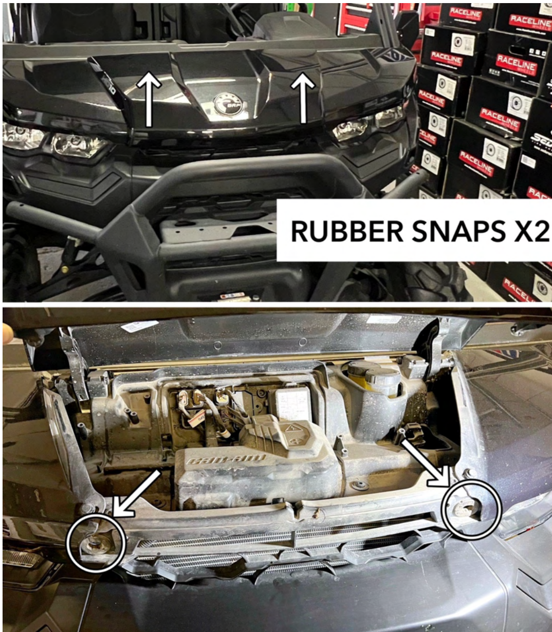
FIGURE 1: HOOD REMOVAL "PULL HOOD OUTWARD & UP"
