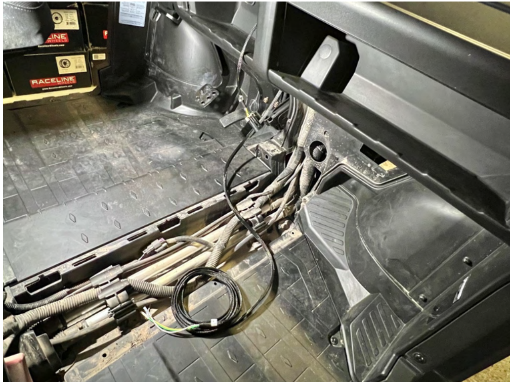
FIGURE 1:2: REAR HARNESS TO MAIN FACTORY PLUG AT REAR OF MACHINE
