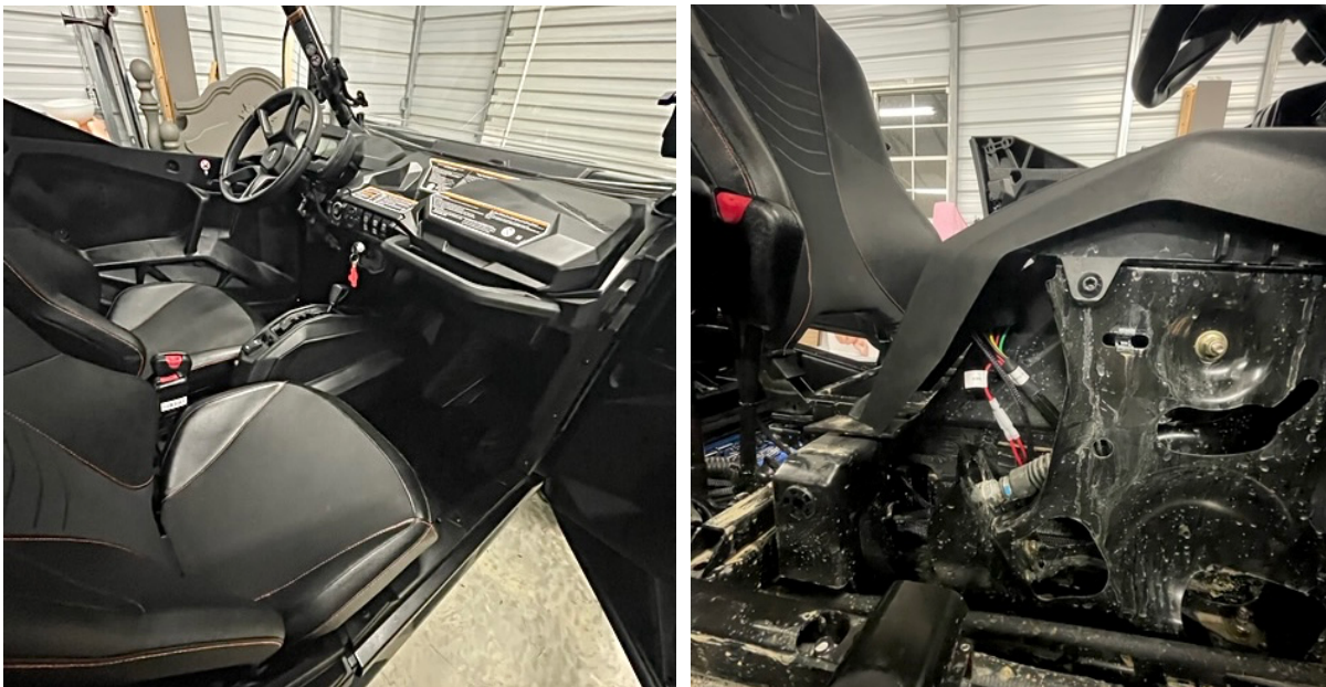
FIGURE 1: START BY REMOVING PASSENGERS SIDE PANEL OF CENTER CONSOLE
