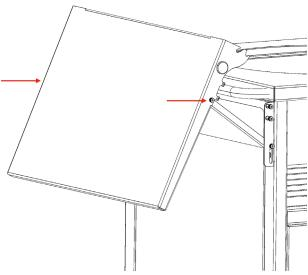
4. To lock the shelf in place, pull the shelf / strut assembly up, and pivot the shelf down and onto the shelf pins. The shelf should sit firmly on the pins, and with the strut fully lowered in the bracket slot.
