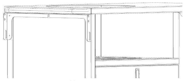
2. Secure in place first with one (1) of the supplied self-tapping sheet metal screws in the center of the bracket to the underside of the countertop. Then secure to the sides with the remaining four (4) screws.
