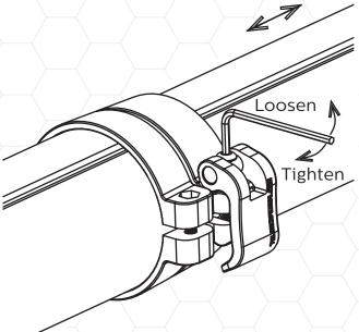
Clamp bolt needs to be adjusted so the smaller tube does not slide when clamp is closed (as shown). The tube should slide easily when the clamp is open.
