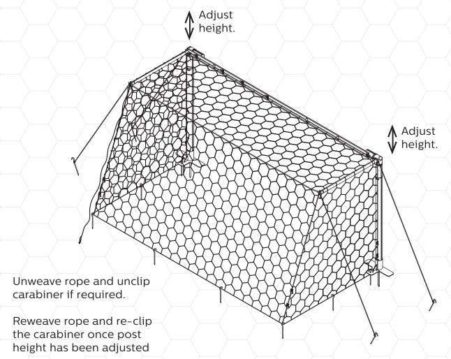
Remove ground pegs holding nets in place. Peg once the post height has been adjusted.
