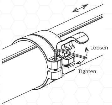
To ensure the plastic clamp connector is secured to the large tube, tighten the bolt with the 3/32 allen key, ensuring the smaller tube slides easily with the clamp open as shown.
